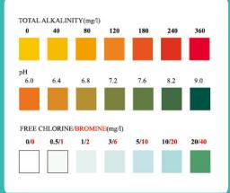
Simply dip the strip into the water for 2 seconds and then remove it immediately. Hold horizontally for 60 seconds without removing excess water from strip, and then compare the result against the color chart. You now know if your water needs treatment. Apply treatment, if necessary, and retest before using.
